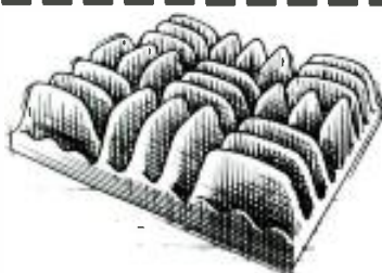
Figure 1. An audio spectrum display shows the spectral distribution of the numerous fundamental frequencies in a multitone signal.
